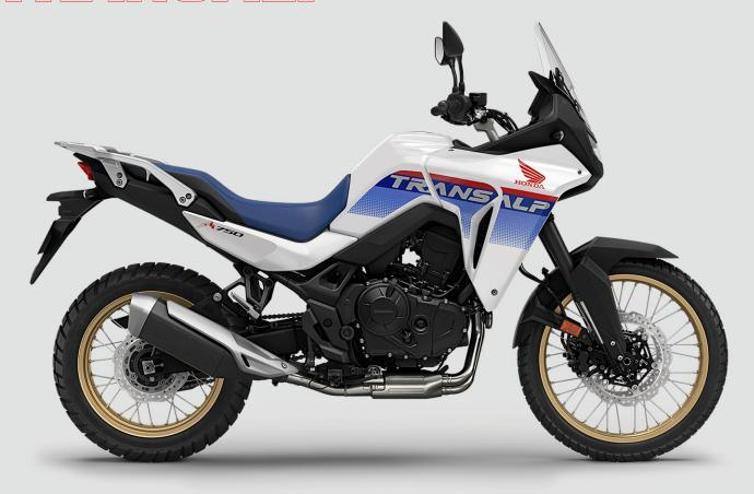
Type: 4-stroke, OHC, Unicam® Displacement: 755 cc, parallel twin-cylinder, 4 valves per cylinder Cooling: liquid
