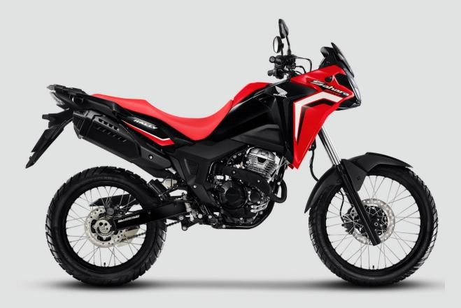
Type: 4-stroke, single-cylinder, OHC Displacement: 293.55 cc Cooling: air-cooled Maximum power: 24.8 hp @ 7,500 rpm Torque: 19.5 lb-ft @ 5,750 rpm (26.4 Nm)
