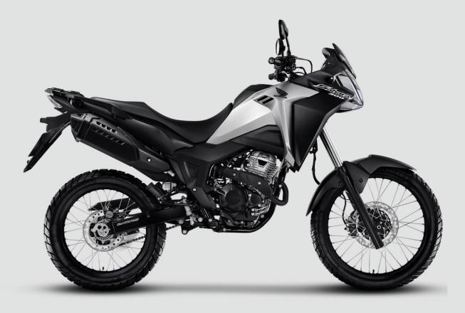
Type: 4-stroke, single-cylinder, OHC Displacement: 293.55 cc Coolina: air Maximum power: 24.8 hp @ 7,500 rpm Torque: 19.6 lb-ft @ 5,750 rpm (26.5 Nm)
