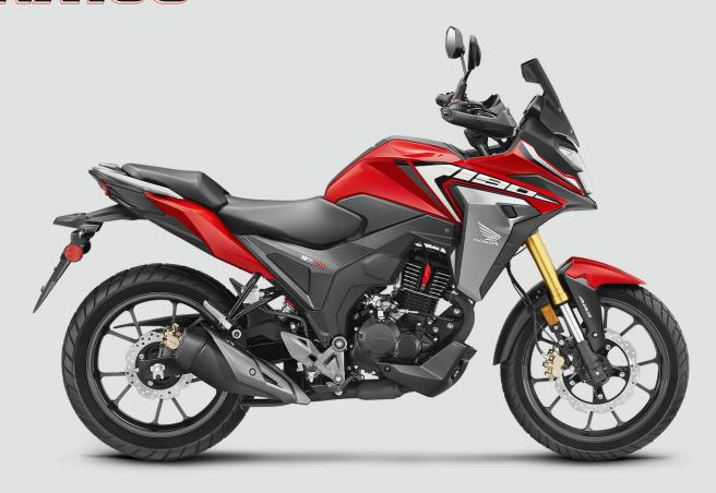
Type: 4-stroke, SOHC SI Displacement: 184.4 cc, single-cylinder, 2 valves Cooling: air-cooled Max power: 16 hp @ 8,500 rpm Torque: 15.3 Nm @ 6,000 rpm
