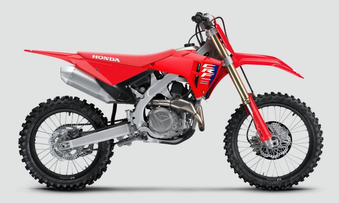
Type: 4-stroke, Unicam® SOHC Displacement: 449 cc, single-cylinder, 4 titanium valves Cooling: liquid
