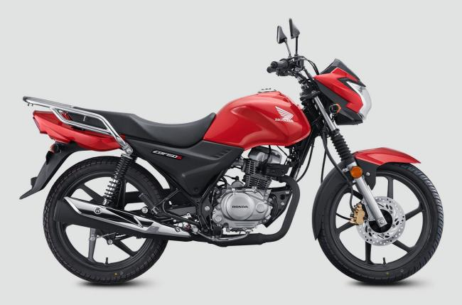
Type: 4-stroke, OHC Displacement: 149 cc, single-cylinder, 2 valves Cooling: air-cooled Maximum power: 11.4 hp @ 8,000 rpm Torque: 11.7 Nm @ 5,500 rpm
